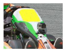
The mounting position on the front panel is fixed horizontally, in the middle axis, and a minimum 10 cm below the bottom edge of the number area of the panel. The camera should not block the view of the number from the front.
